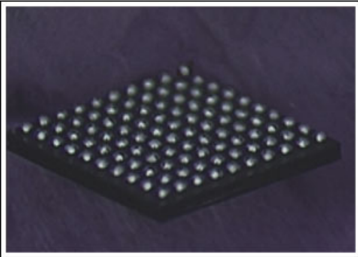
Figure 1. Photo of a 10 x 10 WLP with circuit side view
